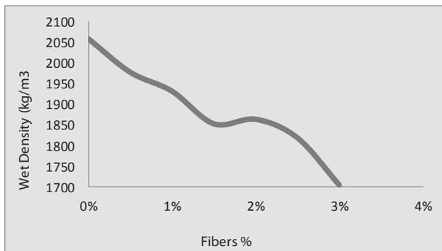
**Fig.(3): Wet density of mortar.**
