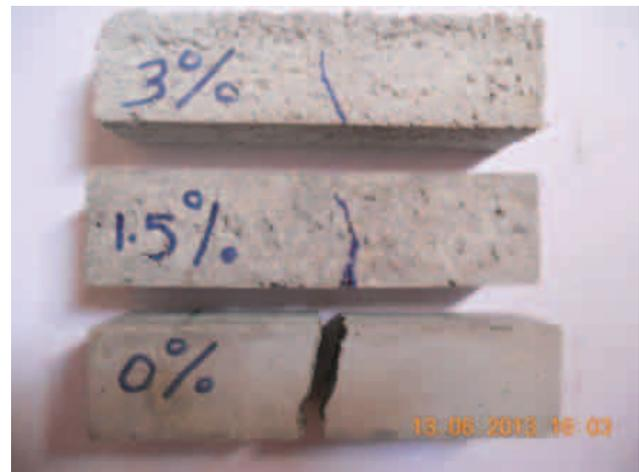
**Fig.(10):** Failure modes of mortar after flexural strength test.
