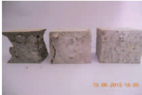
**Fig.(8):** Failure modes of mortar after compressive strength test, the left sample is for original mix, the middle is for mix with 1.5% fibers and the right one is for mix with 3% fibers.
