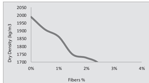
**Fig.(4): Dry density of mortar.**
