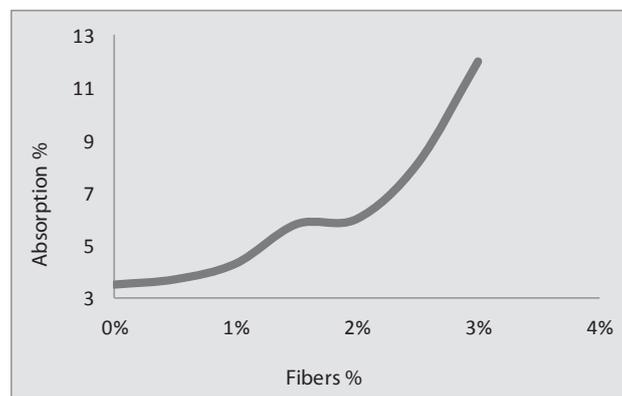
**Fig.(5): Water absorption of mortar.**
