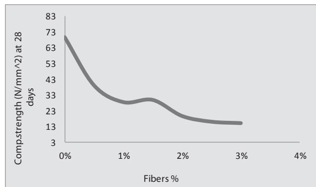
**Fig.(7): Compressive strength at 28 days.**
