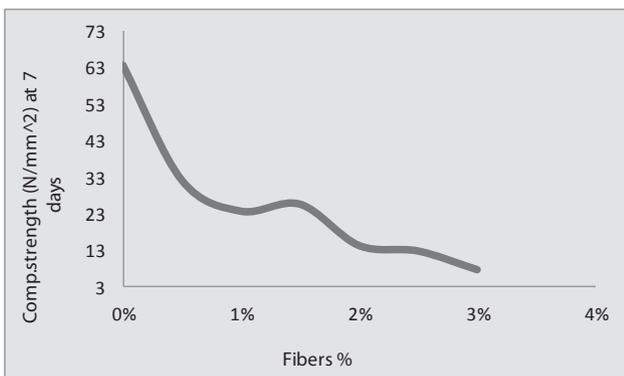
**Fig.(6): Strength at 7 days compressive.**
